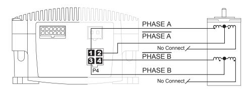
Figure 2.3.4: 6 Lead Half Coil (Higher Speed) Motor Connections
